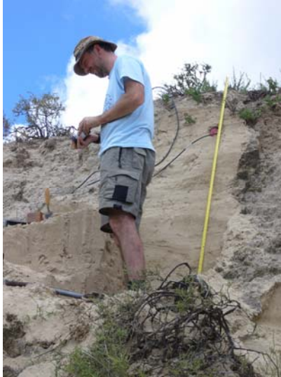
Mark Bateman of the University of Sheffield seals a sediment sample extracted from a pan fringing lunette dune in the western Free State. Sampling every 50 cm down the profile will hopefully provide good temporal resolution in terms of late Quaternary aeolian activity in this part of the Free State.
